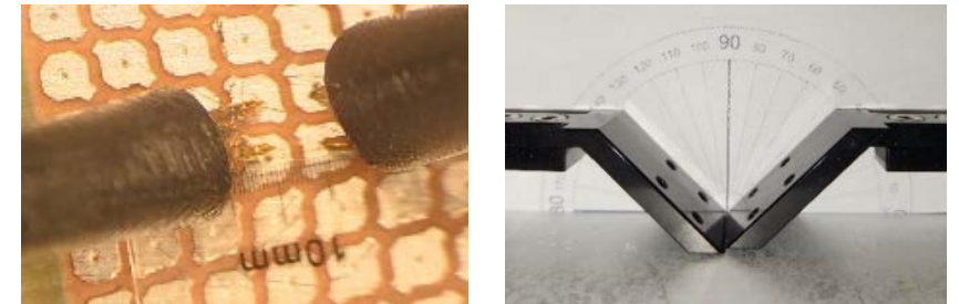
(Left) probe landing spacing measured. (Right) 45 degree probe landing angle used.
