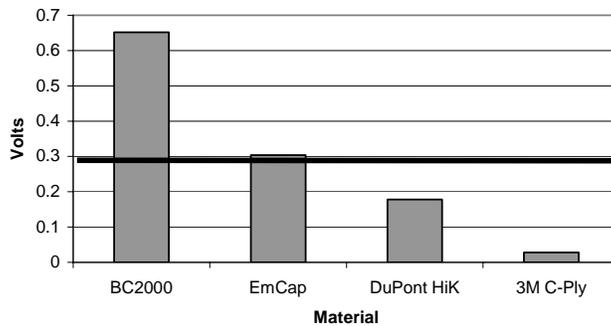
Figure 2-4. Peak-to-peak Voltage Between Vcc and Ground in 4-up Configuration
