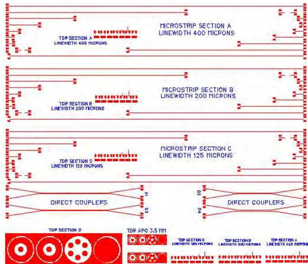
Figure 1-2. High-Frequency Test Vehicle Layer 1 Artwork
