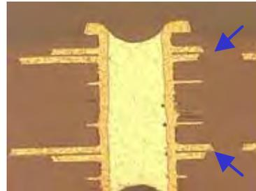
C-Ply cores separated by regular core.
