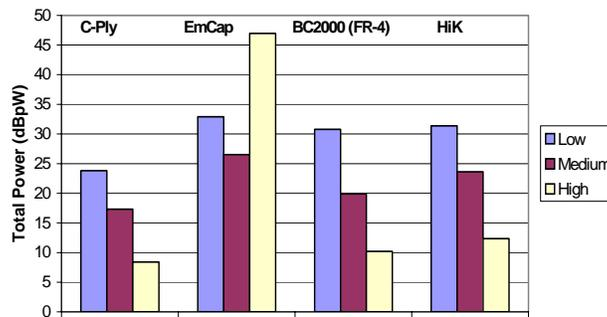
Figure 2-8. Comparison of Common-mode Noise on TV1-4-1 With No Decoupling Capacitors
