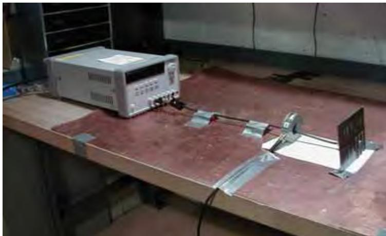
Figure 2-5. Test Setup for Common-mode Noise Measurements
