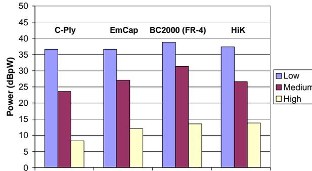
Figure 2-7. Comparison of Common-mode Noise on TV1-1-1 With No Decoupling Capacitors
