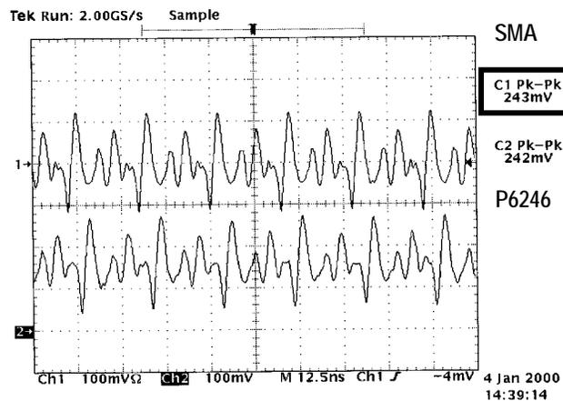
*Figure 2-2. Peak-to-peak Ripple Voltage*
