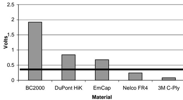
Figure 2-3. Peak-to-peak Voltage Between Vcc and Ground in 1-up Configuration
