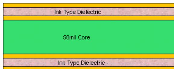
To support open/short test, we designed specific vias to lead out inner ground layer. As shown in the 3D drawing, yellow layers represent copper layers; grey layers represent ink type dielectric, and the green layer represents FR4 core.
