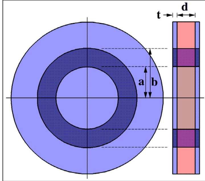
Figure 1: Radial Transmission Line Cross Section
