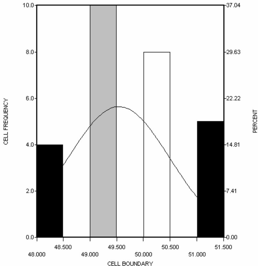
Fitted curve is a Normal. K-S test: 0.200. Lack of fit is not significant.
