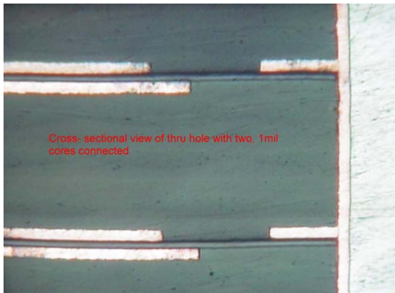
Figure 2: Cross sectional view of through hole with two 1-mil cores connected
