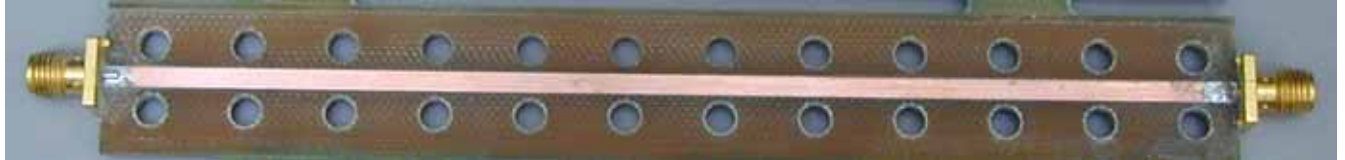
Figure 2.: Photo of the scaled test structure with edge-launch SMA connectors at its ends.
