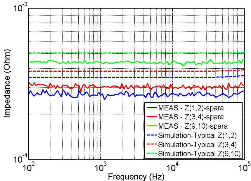
*Figure 13. Measured and simulated self-impedance of the board with shorts at capacitors*
