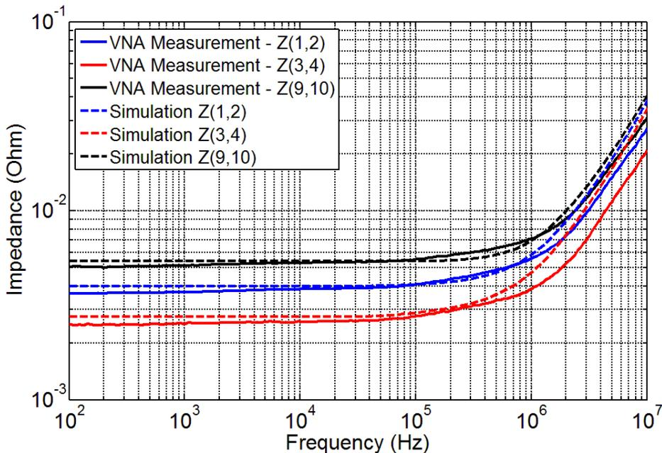
**Figure 10.** Self-impedance results of measurements and simulations of the board with shorted DC-DC converter pads
