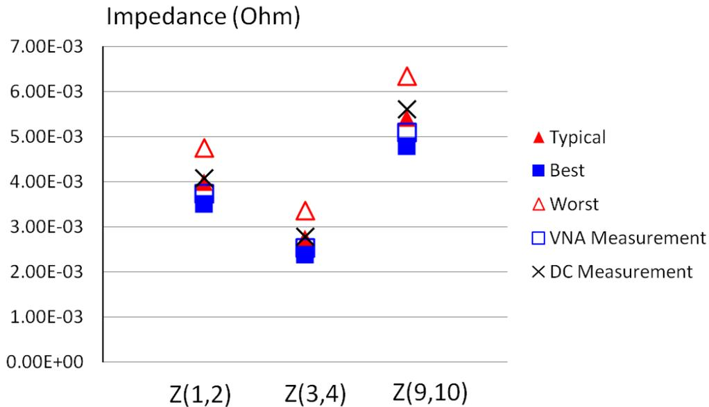
Figure 8. Typical, best, and worst case self-impedance results of simulation closely correlate with low-frequency VNA and DC measurements.
