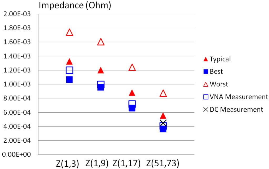
*Figure 9. Transfer-impedance simulation and measurement results of typical, best, and worst case at 1mOhm and below.*
