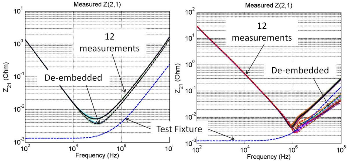
**Figure 13.** Measured impedance of 12 capacitors and test fixture together with de-embedded models. 1000uF (left) and 47uF (right) capacitors.
