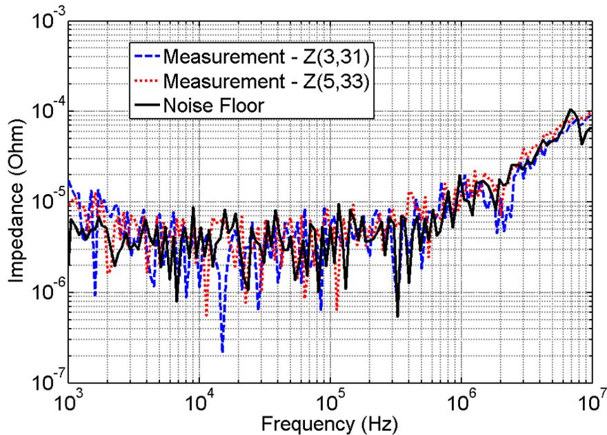
*Figure 4. Noise floor of the measurement system with two transfer impedances not being recognizably above the noise floor.*
