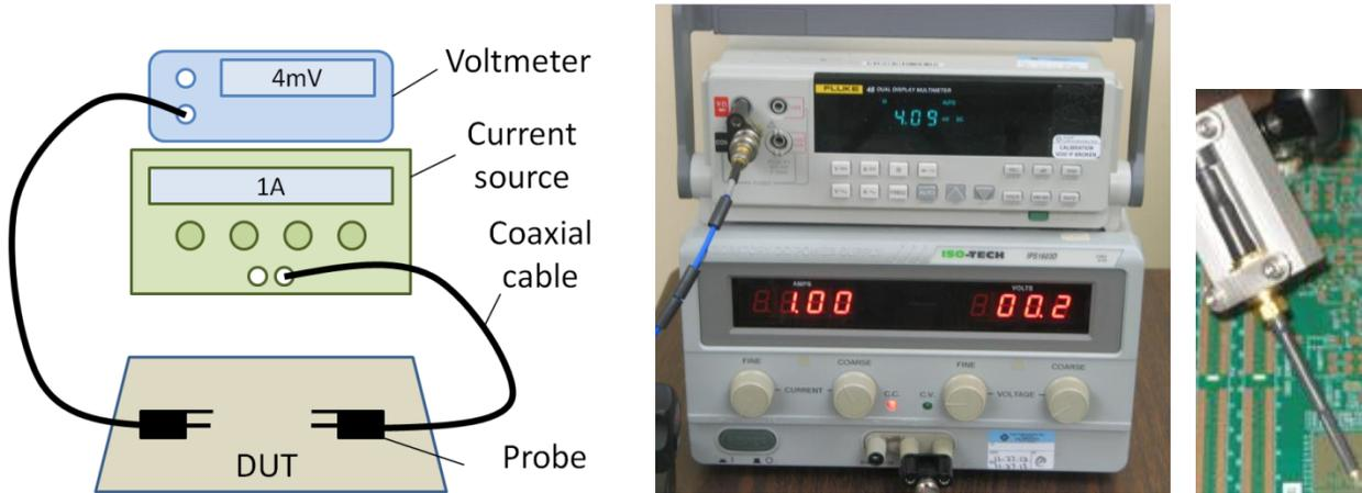
*Figure 5. DC measurement setup sketch on the left, photo of actual instrumentation in the middle, home-made semirigid probe in 3D holder on the right.*
