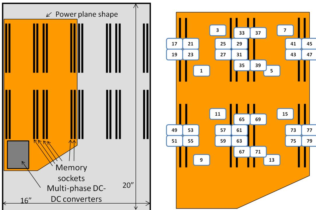
*Figure 3.* Sketch outline of a large printed circuit board with multiple memory sockets. The left side shows the approximate dimensions and placements, the right side shows the port-numbering definition.
