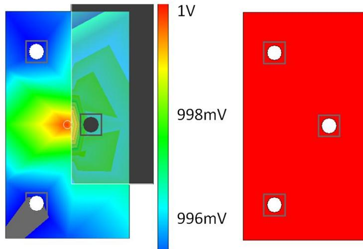
*Figure 1.* DC drop on a large surface pad with default-size node connection (left) and equipotential pad option (on the right).
