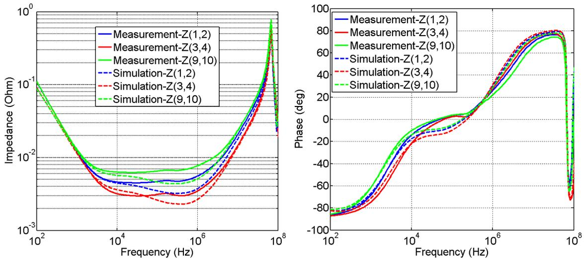
**Figure 14.** Self-impedances from simulations and measurements of the capacitor loaded DUT.
