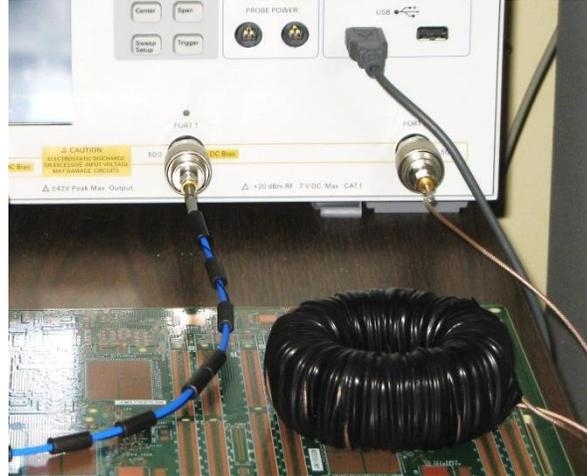
*Figure 6. AC measurement setup with regular two-port VNA and ferrite toroid common-mode choke.*
