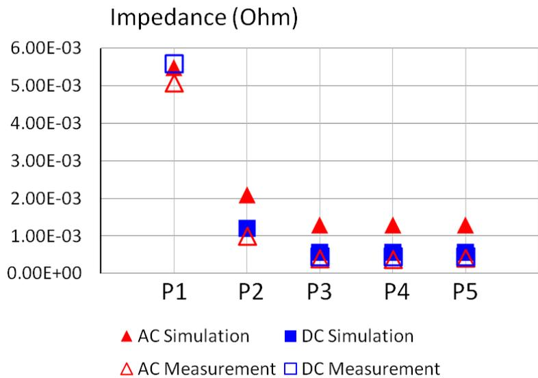
**Figure 2.** Correlation of various measured and simulated responses at low frequencies.
