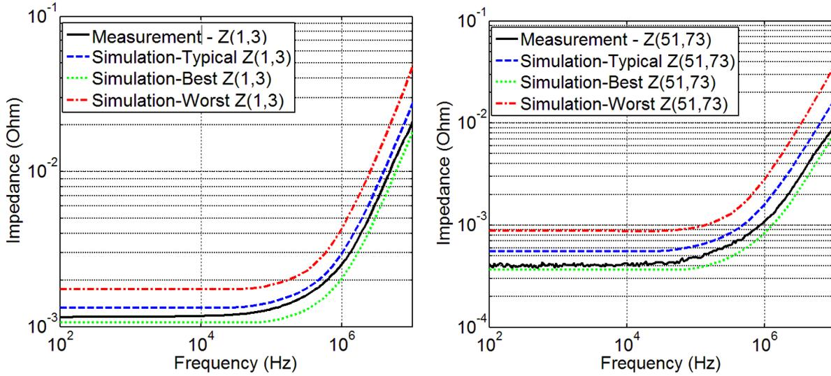
**Figure 12.** Measurement result compared to simulation results with cross-section data.
