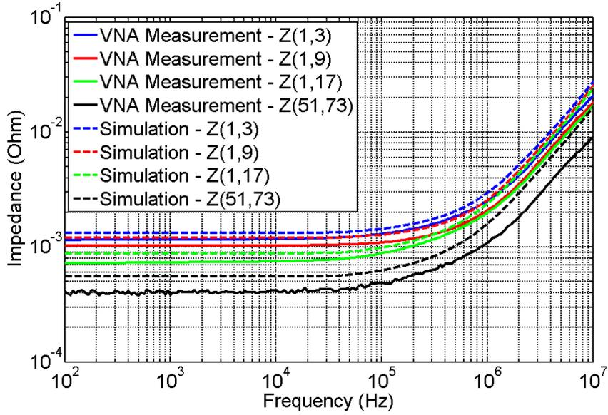
**Figure 11.** Transfer-impedances from measurements and simulations of the board with shorted DC-DC converter pads
