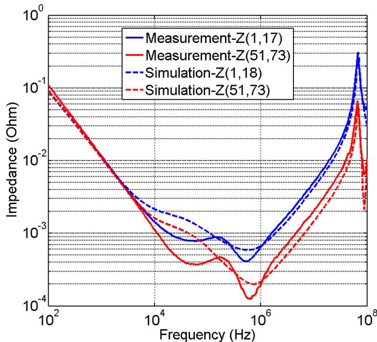
**Figure 15.** Transfer-impedances from simulations and measurements of the capacitor loaded DUT.
