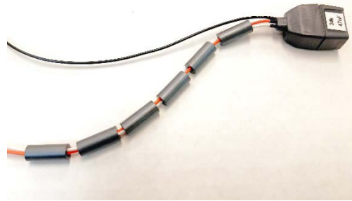
Figure 13: Noise suppression with ferrite beads on the sense wires.
