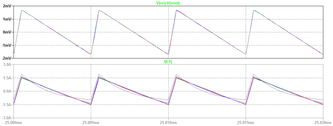
Figure 8: Impact of the inductor's resistance on the extracted current-sense voltage (top) and actual inductor current (bottom).
