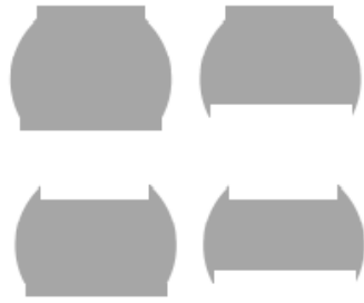
Figure II.10 Real solder ball shapes (reproduced from [II.2])
