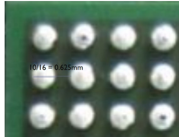
Pre-reflow solder ball
