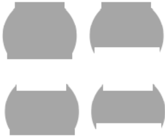
Real solder ball shapes
