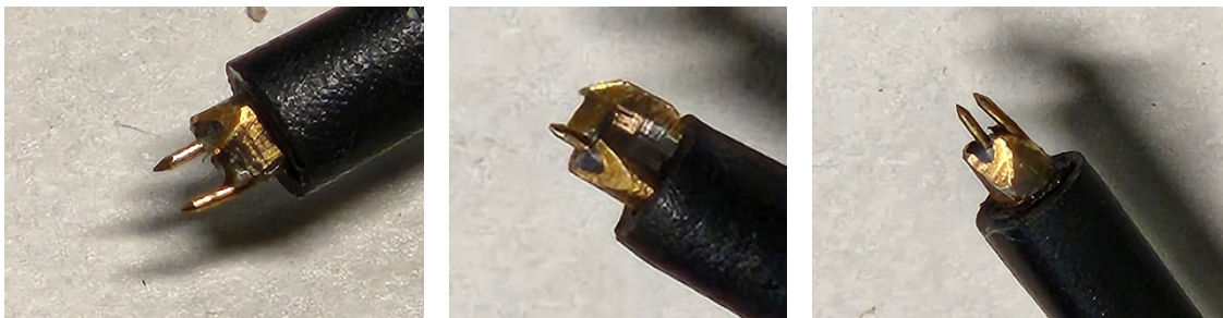
Figure 15: Wafer probes used in the measurements. 1mm pitch RP (left), 1mm pitch SP (mid), 0.5mm RP (right) probes
