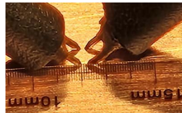
(Left) Probe landings for copper sheet impedance measurement.
