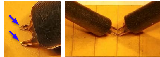
(Left) Deflection of light shows probe touchdown. (Right) Mylar sheet supplied with probes confirm alignment.
