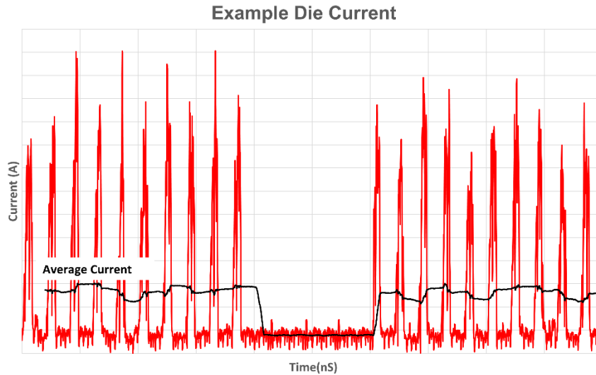
Figure 2: Sample transient current waveform in core PDN at the die vs time averaged current
