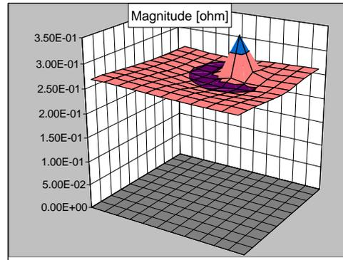
Magnitude of self-impedance (on the left) and transfer-impedance (on the right) plots at 100MHz. The transfer impedance is shown from 3 inches and 4 inches away from the corner, where the peak of the impedance profile occurs.
