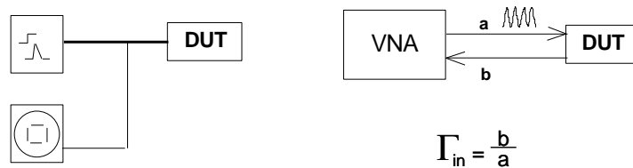
Fig. 1: Block schematic of TDR measurements in the time and frequency domain.
