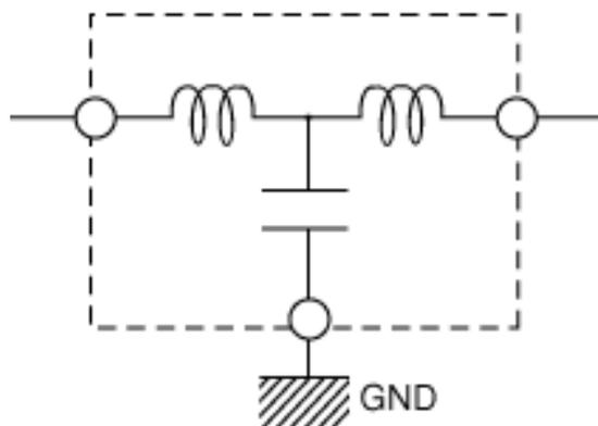
Three-node EMI T filters are optimized for 50-ohm operation.
