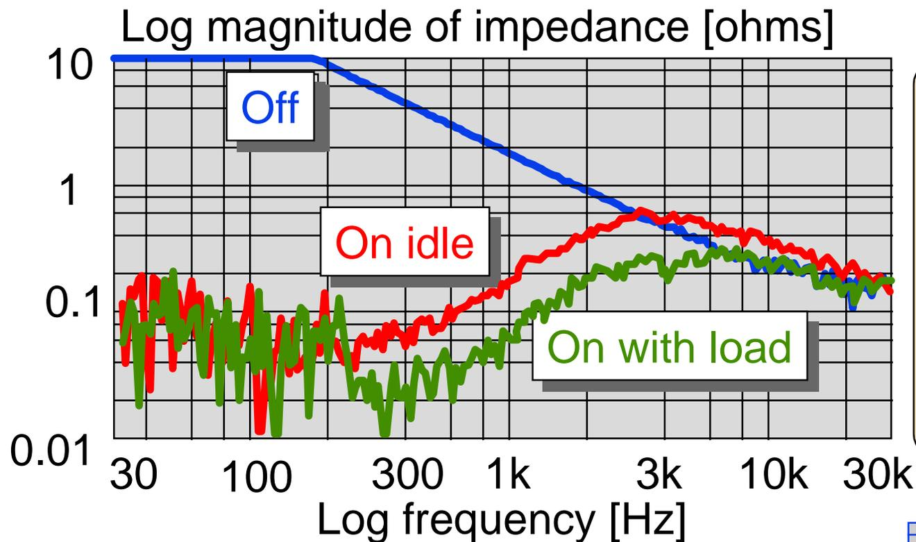
Output impedance varies with input and output conditions ( $V_{in}$ ,  $I_{load}$ )
