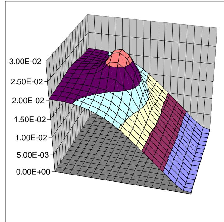
Simulated DC voltage drop on a pair of 3"x3.6" one ounce copper planes, with single-point feed at the front corner (left graph) and with line feed (right graph). Model: resistive grid with 0.2" grid size, 25A DC current sink at 1.5"x1.5" from upper left corner.
