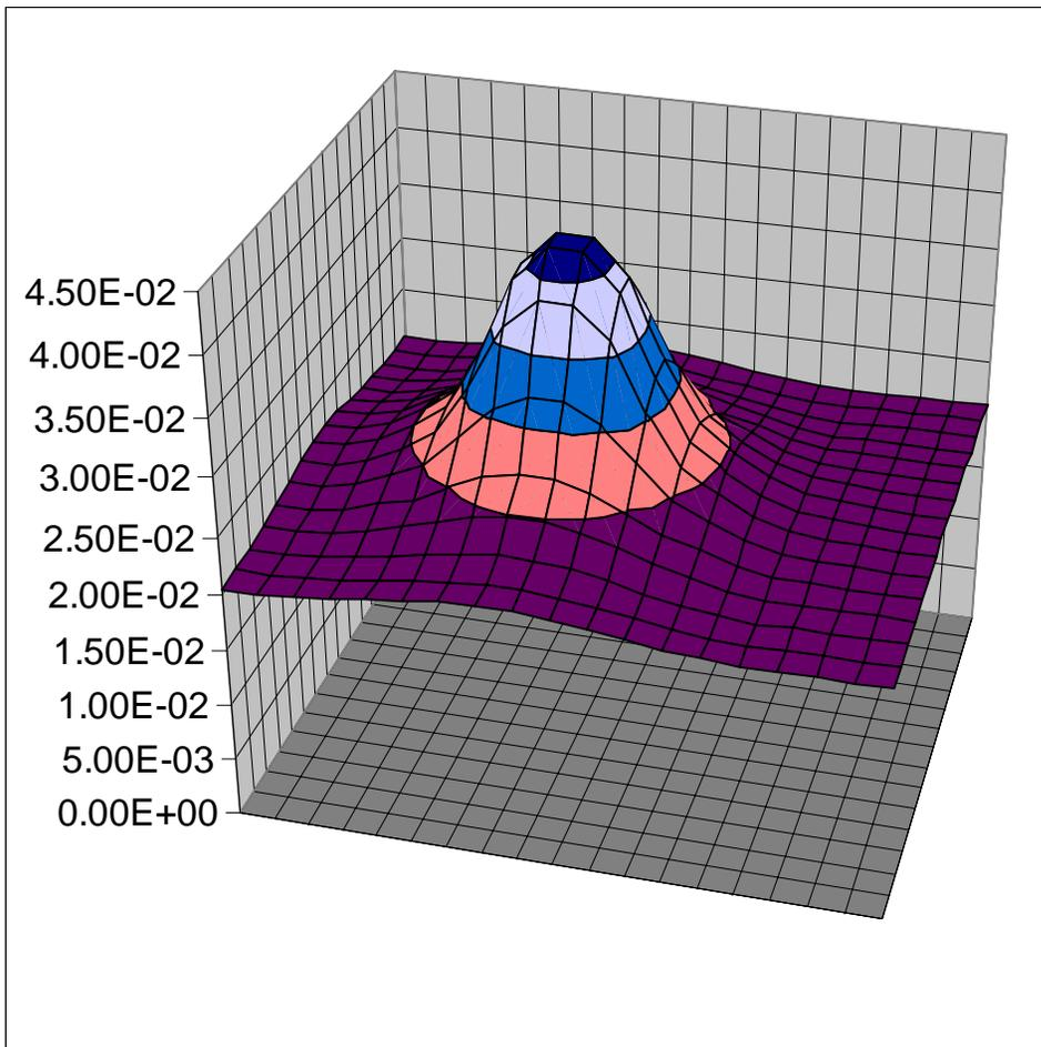
Simulated inductive voltage drop (mV) on a pair of 3"x3.6" copper planes with 1mil separation. Model: Tline grid with 0.2" grid size, 2A/nsec PWL current sink at 1.5"x1.5" from upper left corner.
