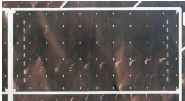
Figure 1. Etched C-Ply layer for Sun test board.
