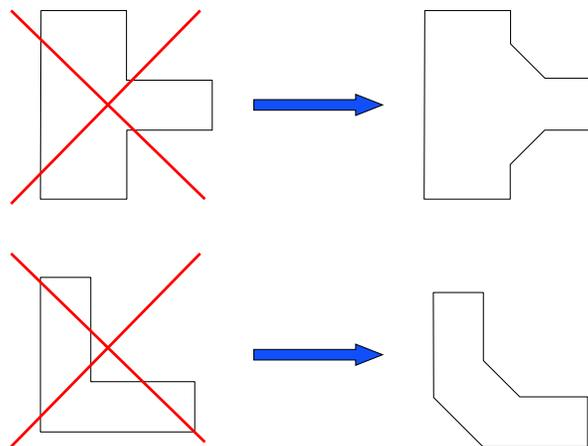
*Figure 8: Suggested geometries to avoid current crowding at sharp corners.*
