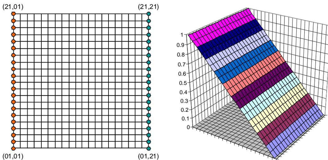
*Figure 4: Berkeley SPICE model to simulate the current flow in square plane shapes (left) and potential surface (on the right).*
