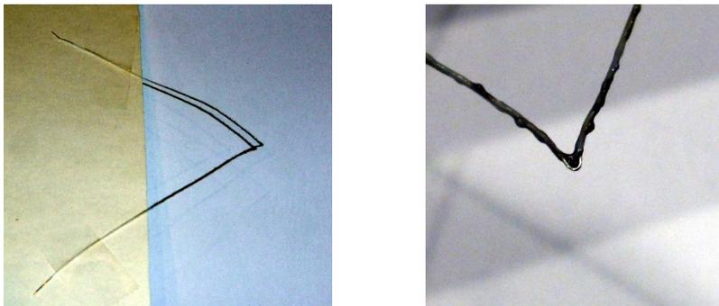
*Figure 1: 30-gauge solid wire mounted at the edge of a cardboard sheet with (originally) white insulation with a sharp bend in the middle, after exposed to several ampere of DC current. Left: full view; right: close-up of the bend.*
