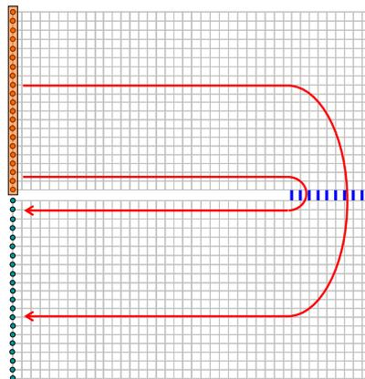
*Figure 7: SPICE circuit representation with the shortest and with a longer current path marked by red lines.*
