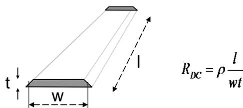
*Figure 2: Cross section and resistance calculation of a PCB trace.*
