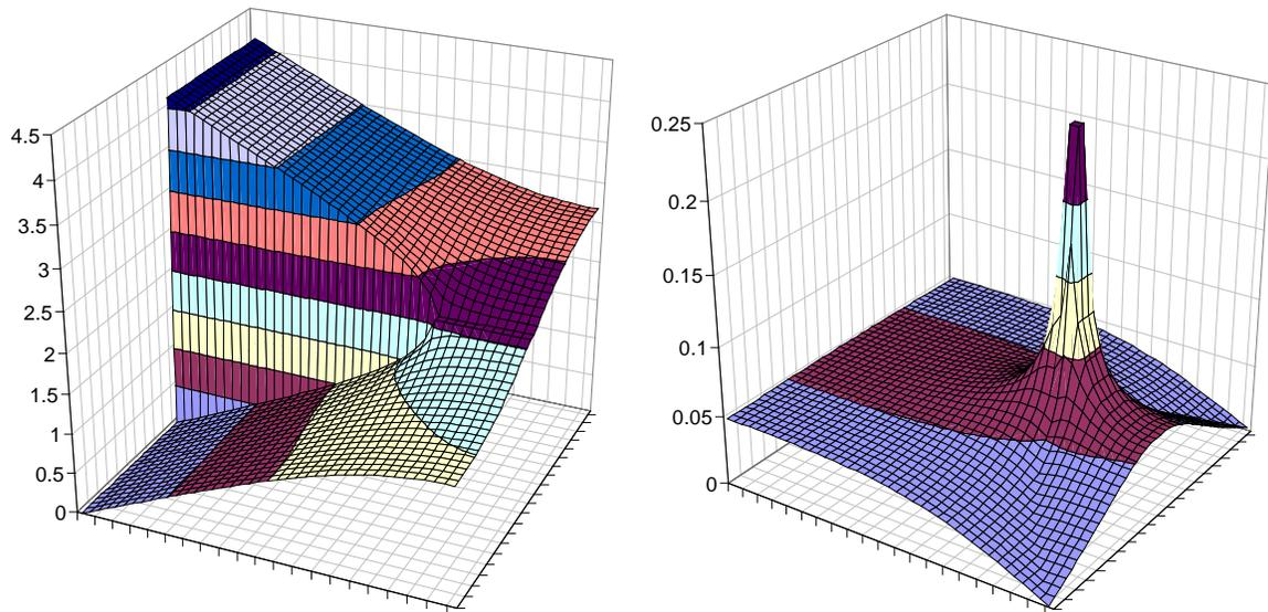
*Figure 6: Potential surface (on the current) and relative current density (on the right) of the circuit shown in Figure 5.*
