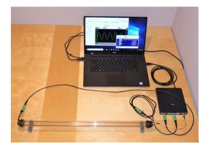
This image above shows a newer TiePie oscilloscope model, HS5, with 500Ms/s sampling speed and 1uHz-40MHz arbitrary waveform generator, shown here as I prepare one of the transmission-line illustrations for my SI training courses.
