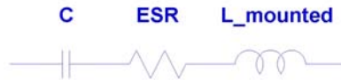
Figure 3: A possible equivalent circuit for the bypass capacitor, using the mounted inductance
