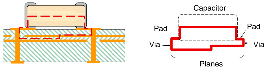
Figure 1: On the left: side cross section view of a mounted bypass capacitor. On the right: contributors to the loop inductance. The red line represents the current loop.
